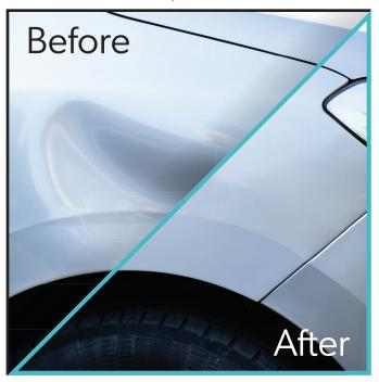
Our Paintless Dent Repair process involves manipulating the metal back into its original shape without the need for sanding, filling, or repainting. This repair method is faster, less expensive, and does not compromise the original paint finish... making it the optimal solution for minor cosmetic damage on vehicles.
